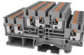
2.5mm 2 Double level Terminal Block, 3 connection poles on each level
